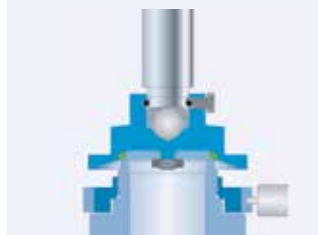
O-ring disc J21: CR "K" J22: EPDM "D" J23: FKM "L" J20: FFKM "C"
