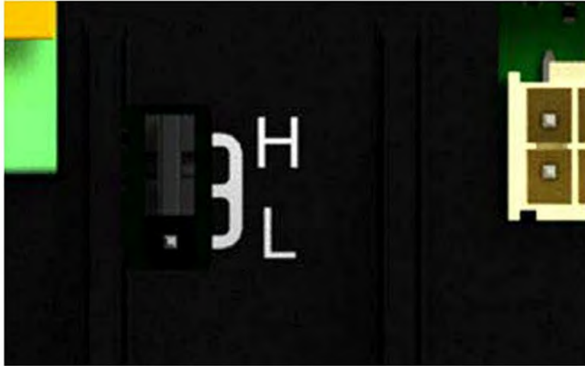
Figure 2: Loop Current Alarm High/Low Selection
