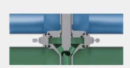
In the radial sealed double-seat valves type R and MX, the lower valve disc opens downward.
