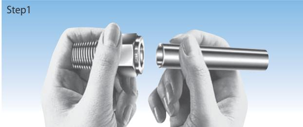
Insert the tubing into the DK-Lok tube fitting until the tubing end bottoms on the shoulder of the fitting body.
