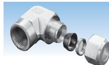
Carbon steel fittings are white zinc plated. Every carbon steel fitting is supplied with SS316 back ferrule and Carbon Steel front ferrule with black fast plated.
