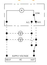
Dotted line indicates wiring by customer.
