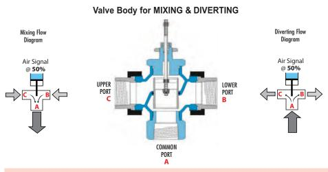
CAUTION: 3-Way Valves are not designed for use in steam applications.
