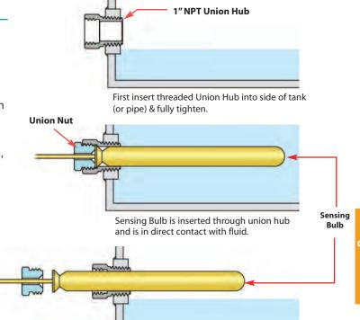
Liquid level must be lowered below sensing bulb insertion point for installation or removal.
