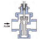
**Normally Open Valves** are used for **HEATING**, so the valve stem closes (**in-to-close**) as the control signal (temperature) increases.
