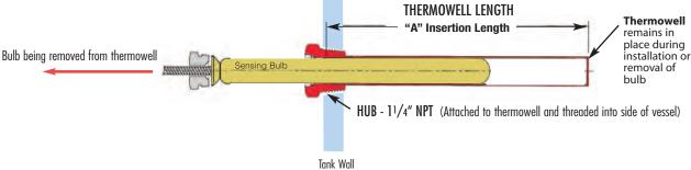
\*Note: Bulb diameter for 9" Bulb is 3/4" and the Union Hub is 1" NPT. For custom 3/4" Union Hub, consult factory.
