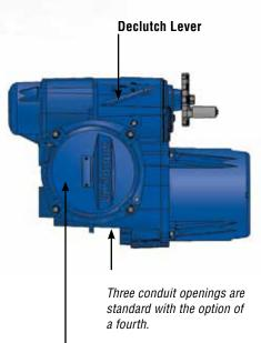
**Terminal Compartment** with O-ring seals that permit a double-sealed compartment, isolating the electronic controls from the environment.
