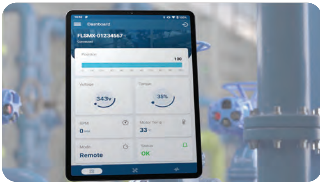
Immediately identify conditions or issues by viewing actuator status and RPMs along with temperature measurements. Confirm the actuator's position and check its voltage and torque.
