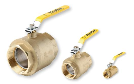
Flow-Tek's Series 51 brass ball valves are the ideal utility valve for low pressure commercial applications. The two-piece body construction offers simple quarter turn operation, low operating torque and bottom entry blowout proof stems. The balls are hard chromium plated brass for added durability and longevity. The Series 51's full port design minimizes pressure drops while maximizing flow.
