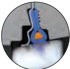
No line pressure. (Pre-fire event condition.)
