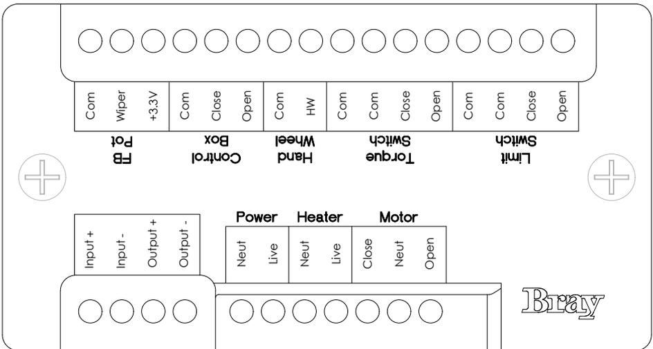
Figure 11: 120VAC / 230VAC Servo NXT terminal labels
