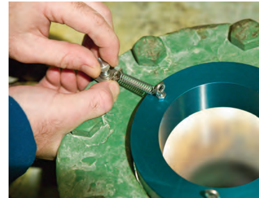
Simple installation. The Phaeton XTL clips on in two minutes or less.
