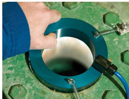
Cool operation eliminates "baked-on" product blocking the window.
