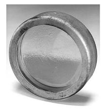
Borosilicate glass under attack by caustic
