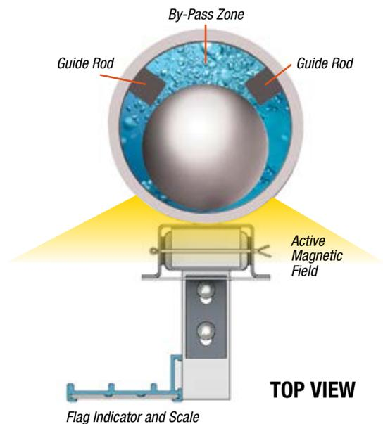
**Note:** The indicator orientation must be specified at the time of order placement. Indicator cannot be rotated beyond active magnetic field during placement.
