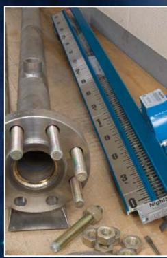
NightStar® Indicators can be field-upgraded on any Jerguson® magnetic indicator, or other manufacturer's indicator, by replacing both the float and indicator.
