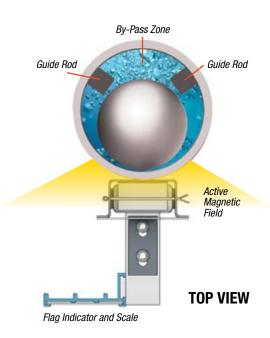
**Note:** The indicator orientation must be specified at the time of order placement. Indicator cannot be rotated beyond active magnetic field during placement.
